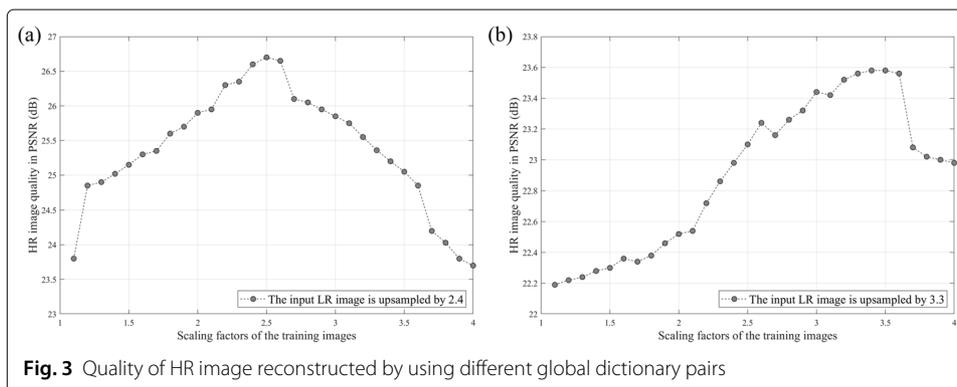
Fig. 3 Quality of HR image reconstructed by using different global dictionary pairs
