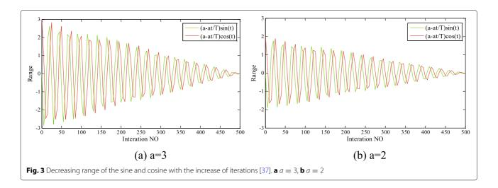
range of sine and cosine is decreased during optimization using Eq. (2) to balance exploration and exploitation.
