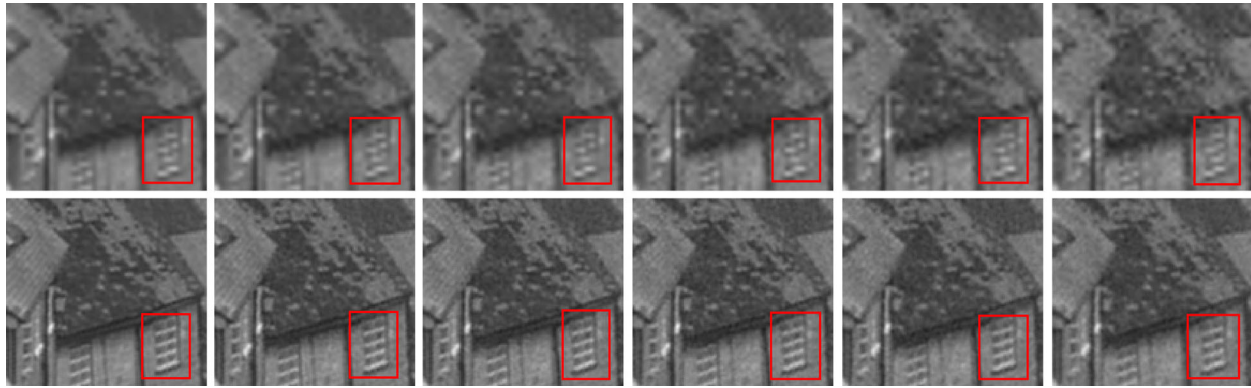
Fig. 1 Reconstructed HR images for different noise levels. Top row: one bicubic-interpolated LR image with up-sampling factor equal to 3 for each noise level, the noise variances are 0, 10, 20, 30, 40, and 50 respectively from left to right. Bottom row: corresponding final HR images reconstructed by OSR with up-sampling factor equal to 3 for each noise level
