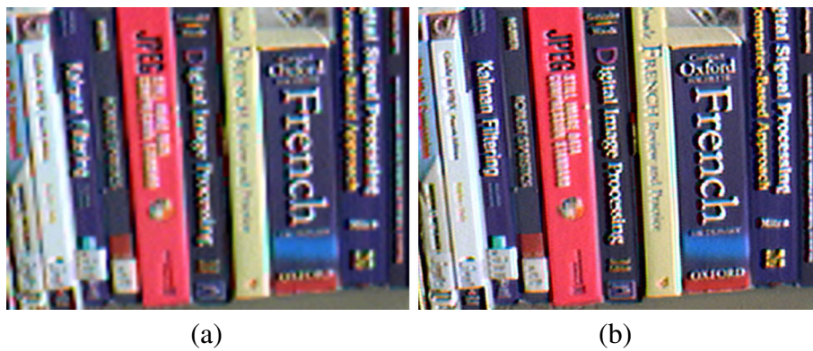
Fig. 7 Super-resolution of bookcase images. a One bicubic-interpolated LR image with an up-sampling scale equal to 4. b Reconstructed HR image by OSR with an up-sampling scale equal to 4
