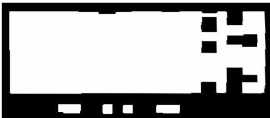
Fig. 8 Closed operation. The closed operation is used to remove the black gap. The closed operator is set according to the condition of the gap
