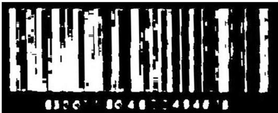
Fig. 7 Image blur processing and binarization. The image is processed in a fuzzy way and two-valued. Processing should pay attention to adjusting the corresponding fuzzification parameters and threshold parameters to get the best results
