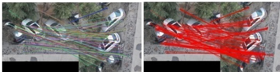
Fig. 11 Effect of the ORB algorithm on the same-scale image feature detection
