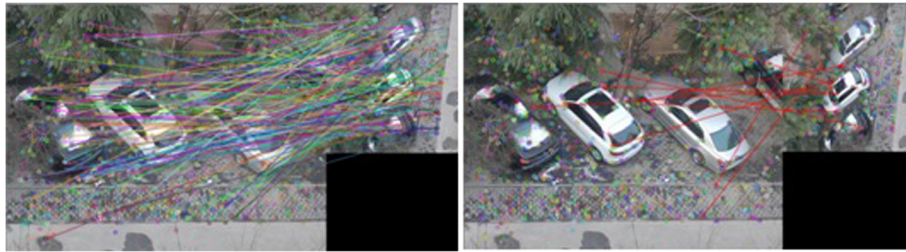
Fig. 18 Results of BRISK algorithm in image detection of different scales
