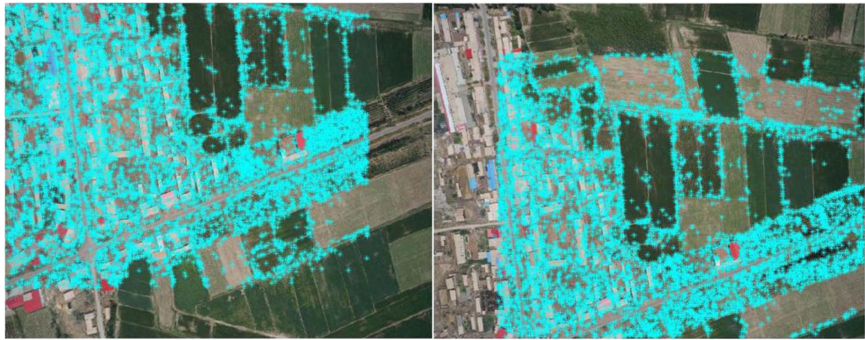
Fig. 3 Feature points extraction using SIFT algorithm and SURF algorithm
