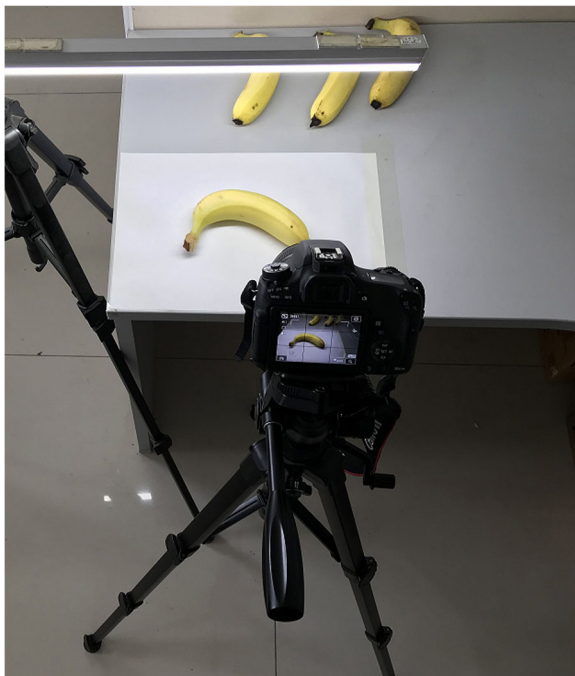
Fig. 2 The proposed computer vision system. The system consists of a camera, a ring fluorescent lamp, the white paper under the banana, and a steady table
