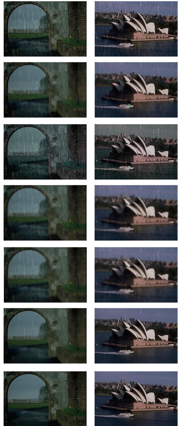
Fig. 5 Comparison of different noising filters for removing raining. The top row is the input rainy images, follows in sequence are the results with Gaussian filter, median filter, bilateral filter, guided filter, the weighted median filter, and the ground true
