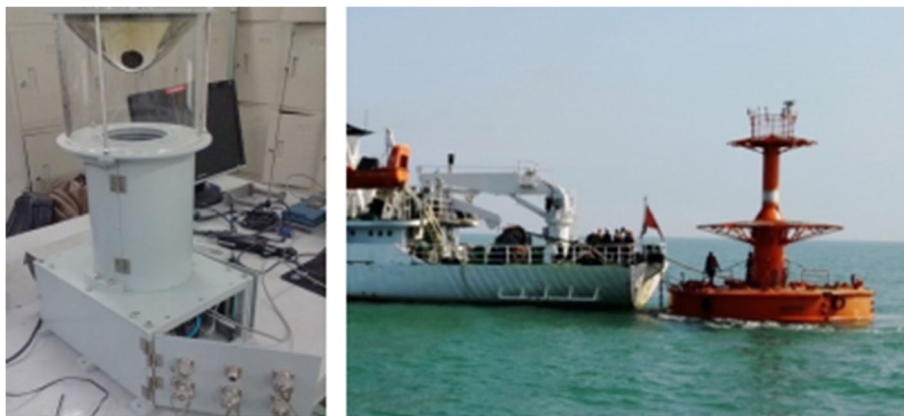
Fig. 7 Equipment. The catadioptric omnidirectional camera (left) and the buoy-mounted omnidirectional system in a marine environment (right)
