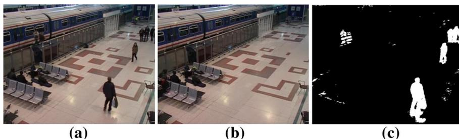
Fig. 2 Moving object detection results. a Original image. b Background. c Segment result
