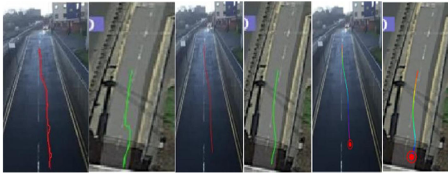
Fig. 19 a Chaotic vehicle trajectory. b Smoothed curve for glyph-based visualization. c Time-stamped semantic glyph representation and lane changes event
