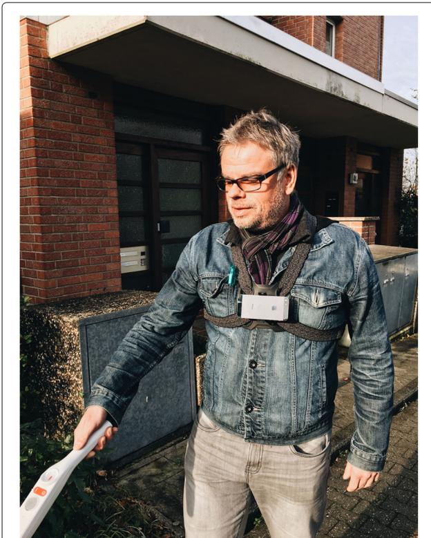
**Fig. 1** Data acquisition and navigation. A smartphone is attached with a chest-mount to the user (*on the left*). For positioning, the user holds an interactive cane, connected to the system via Bluetooth interface and providing navigational clues in a form of a haptic feedback. Data is transferred to a computer using wireless network connection. Consent to use the photograph was obtained
