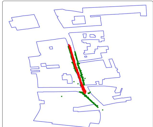
**Fig. 2** Alignment of a model to the OpenStreetMap outline. Green points belong to wall structures; red line is a camera path
