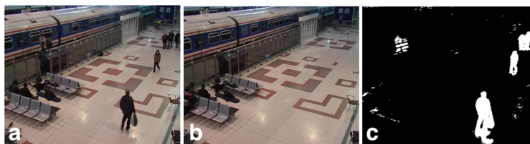
Fig. 4 Moving object detection results. a The original video. b The result for background modeling. c Moving object
