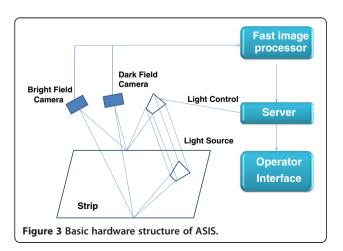
iron and steel plant of China [24]. However, considering maintenance issues and system complexity, most of the systems place the cameras in between the bright field and dark field locations.
