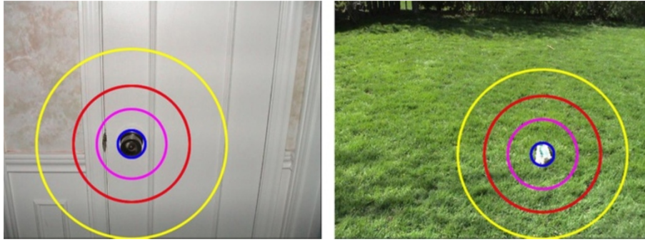
Figure 3 Examples of center regions and surrounding region. Three center regions for the pixel in the circle center are shown, which are the regions within the blue, purple, or red circles. The corresponding surrounding regions are the annular regions between these circles and the outmost yellow circle.
