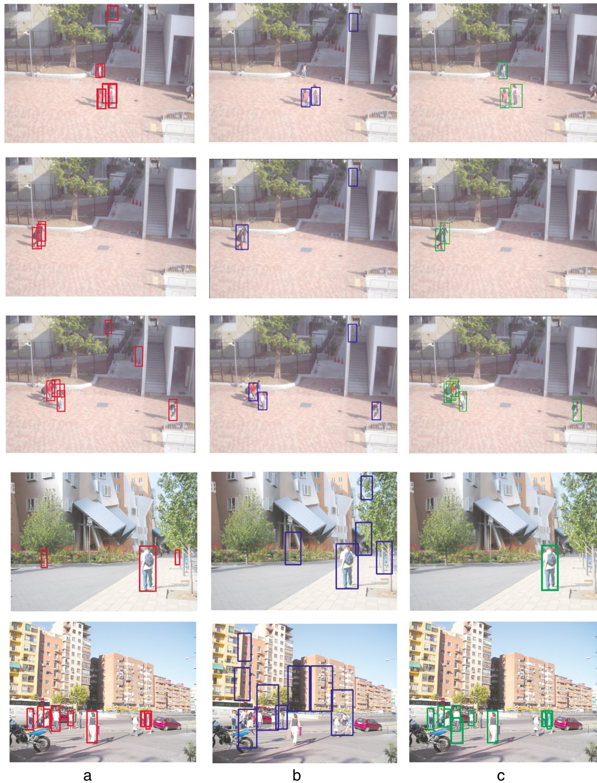
Figure 4 Detection results in outdoor environments. The detection results using the part-based method [11] (a), the voting method [1] (b), and the proposed method (c).
