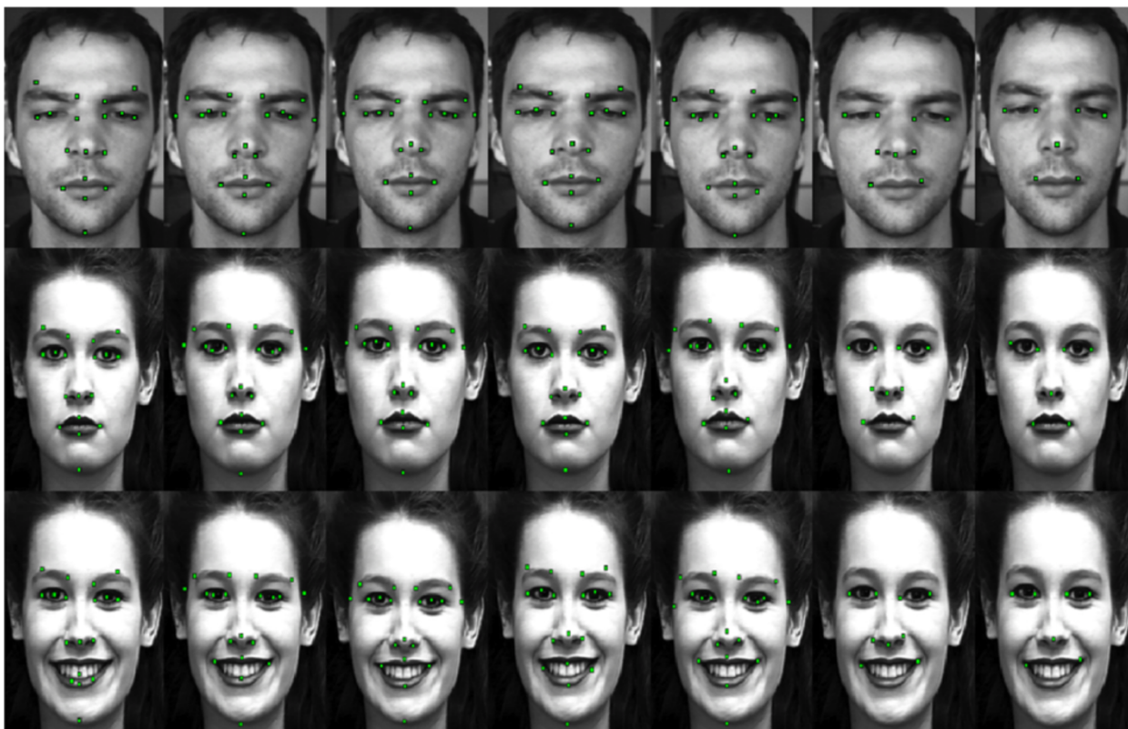
Figure 5 Results of the tested algorithms. The columns refer to different algorithms from left to right: FFPD, AAM, STASM, BORMAN, ZhuRamanan, Everingham, and flandmark. The rows correspond to three different datasets: BioID (upper row), CK+ neutral (middle) and CK+ expressions (lower row).
