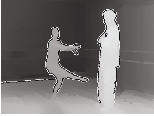
FIGURE 3: Layer Assignment along significant depth discontinuities: foreground boundary layer (black), background boundary layer (white), and main layer (grey values).
