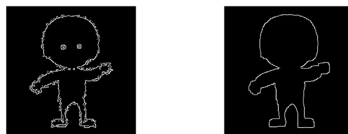
Fig. 12 Extracted contour before and after morphological processing
