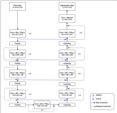
**Fig. 1** 2.5D ResUNet architecture with the slice stack of n = 3. Please note that this diagram is created by the desktop software named diagrams.net (https://app.diagrams.net/), version 14.5.0
