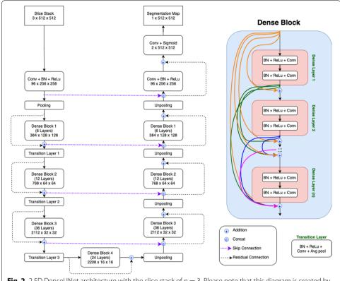
**Fig. 2** 2.5D DenseUNet architecture with the slice stack of n = 3. Please note that this diagram is created by the desktop software named diagrams.net (https://app.diagrams.net/), version 14.5.0
