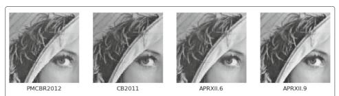
Fig. 19 Fragments of images showing visible artifacts at approximately 1.5 bpp in case of asymmetric scenario of type II
