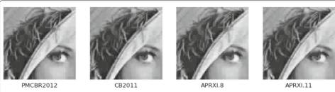
**Fig. 16** Fragments of images showing visible artifacts at approximately 0.3 bpp in case of asymmetric scenario of type I
