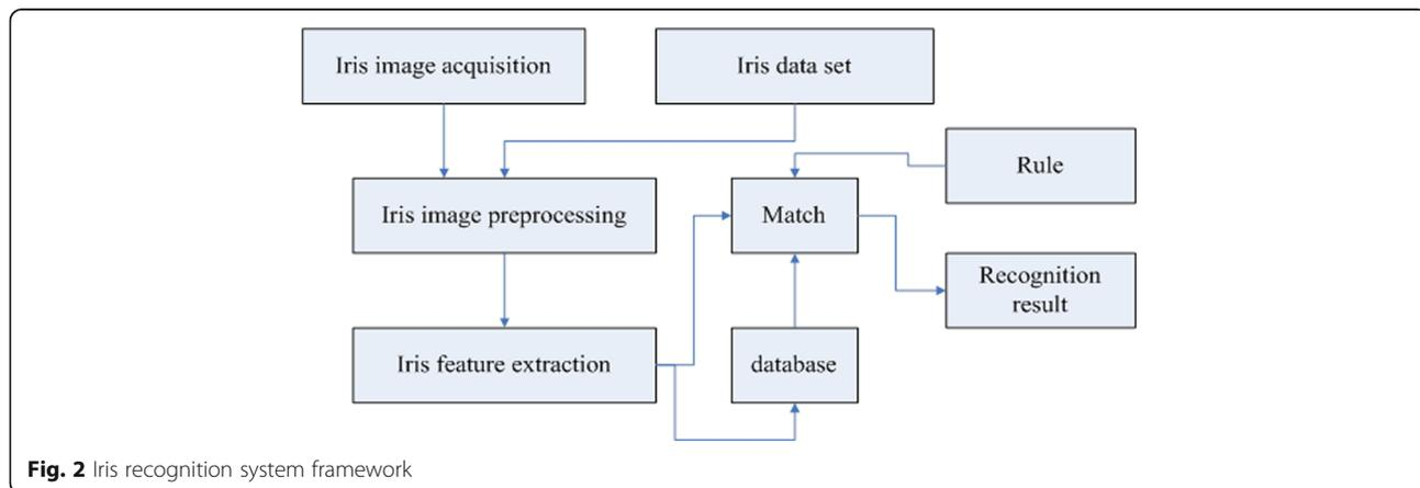
Fig. 2 Iris recognition system framework
