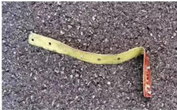
Fig. 1 The twisted metal strip that caused Air France Flight 4590 to crash
