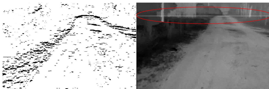
Fig. 18 Vanishing line detection. a Vertical gradient map based on Sobel operator. b Vanishing line detection result
