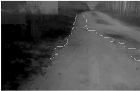
Fig. 10 FCM clustering result based on trapezoid prediction model
