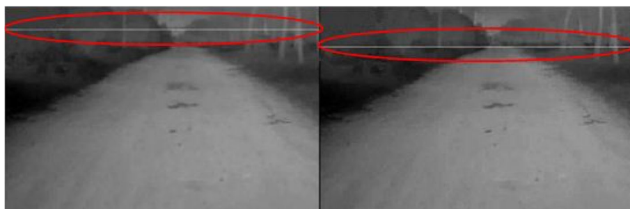
Fig. 19 Result comparison of vanishing line detection. a By Sobel operator and b by normal distribution
