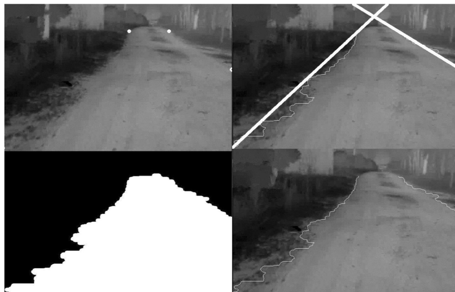
Fig. 4 Trapezoid forecasting model. a Trapezoid vertex figure. b Trapezoid region. c Judged road area map. d Road boundary result
