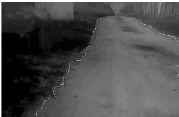
Fig. 11 FCM clustering road boundary recognition result based on probability confidence map
