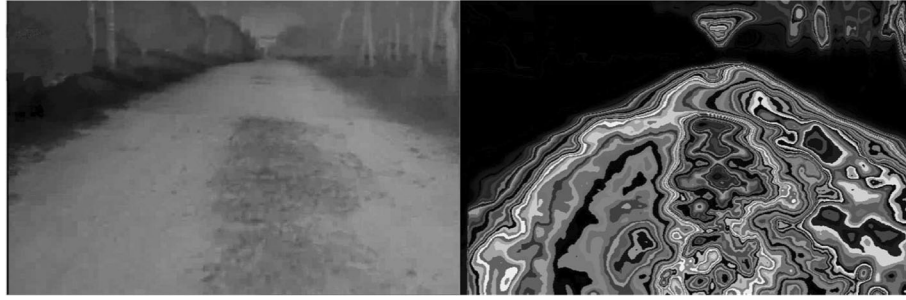
Fig. 13 Backprojection probability map based on road region model. a Original image. b Backprojection probability map
