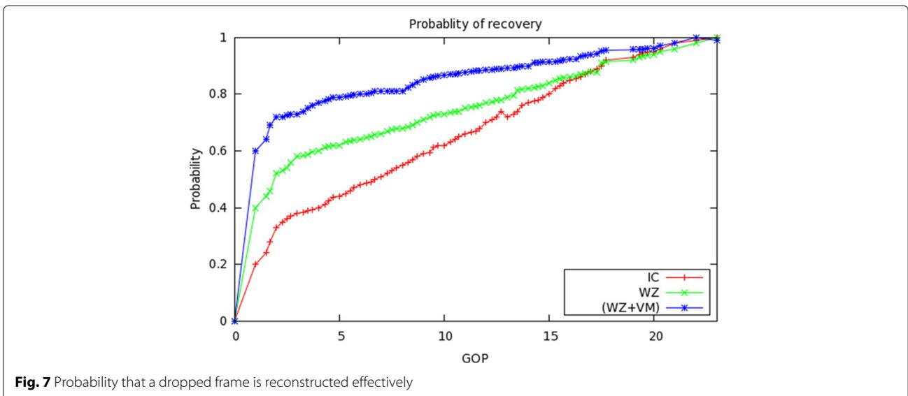
**Fig. 7** Probability that a dropped frame is reconstructed effectively
