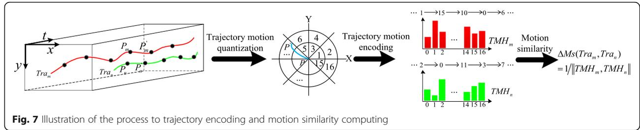
**Fig. 7** Illustration of the process to trajectory encoding and motion similarity computing
