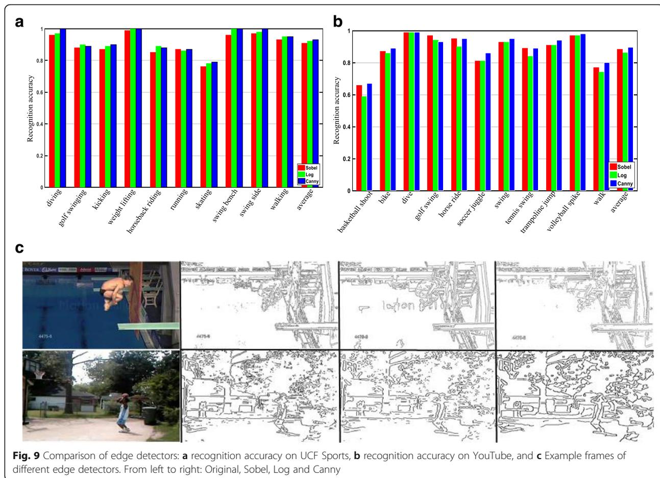
**Fig. 9** Comparison of edge detectors: **a** recognition accuracy on UCF Sports, **b** recognition accuracy on YouTube, and **c** Example frames of different edge detectors. From left to right: Original, Sobel, Log and Canny
