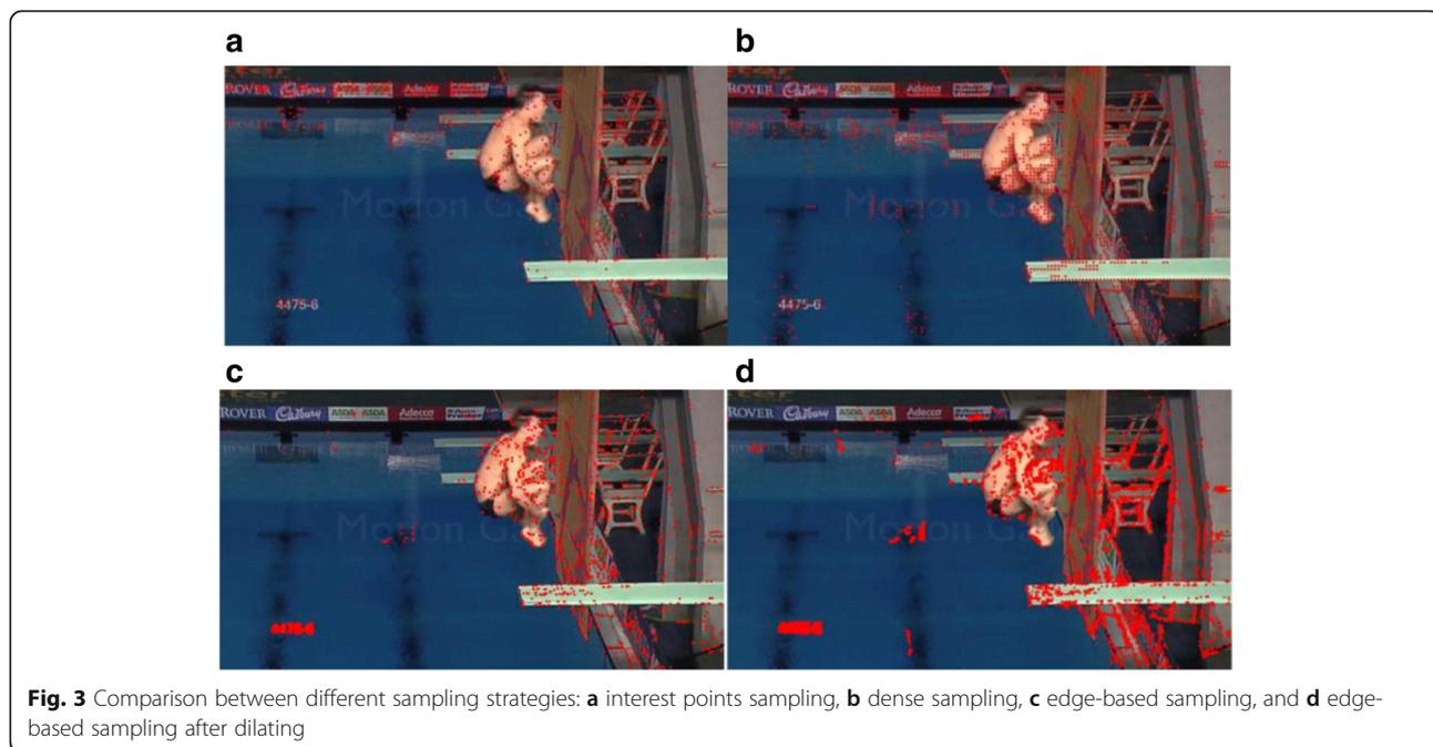
**Fig. 3** Comparison between different sampling strategies: **a** interest points sampling, **b** dense sampling, **c** edge-based sampling, and **d** edge-based sampling after dilating
