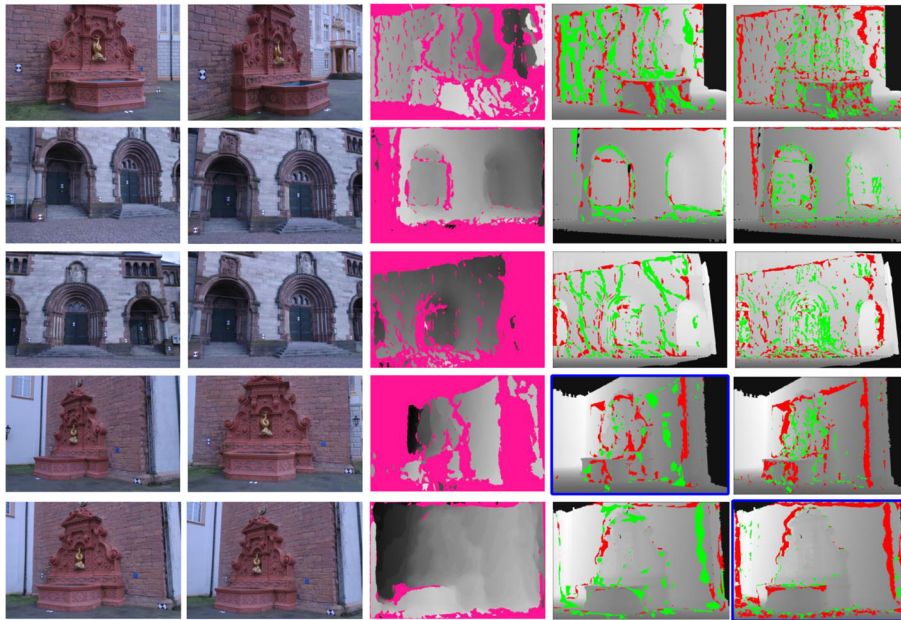
Fig. 9 Representative examples of depth estimation from the Fountain and Herzjesu Dataset. Columns 1 and 2: the stereo pairs. Column 3: depth estimation results by the proposed method, where pink pixels denote occluded pixels. Column 4: comparison of the proposed method with Min et al.'s method [14]. If the depth of a pixel is correctly estimated by the proposed method but incorrectly by Min et al.'s method, the pixel is shown in green color; otherwise, it is shown in red color. Column 5: comparison of the proposed method with the census transform using the same color convention. A blue border around the image indicates the case where the proposed method performs worse compared to the other methods
