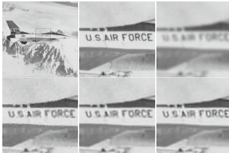
Fig. 3 Deblurring of Jetplane image, scenario 5. From left to right and from top to bottom are the following images: blurred and noisy , fragments of original, blurred, and noisy , results of Fnnmm, IDD-BM3D, and ours. In our method (fixed parameters), the two input parameters, (\sigma, s) , are (7.5, 50) for this scenario, (7.5, 85) for scenario 1, (7.5, 25) for scenario 2, (7.5, 550) for scenario 3, (7.5, 10) for scenario 4, and (7.5, 5) for scenario 6. In our method with automated parameter setting, \sigma_{thr} = 3
