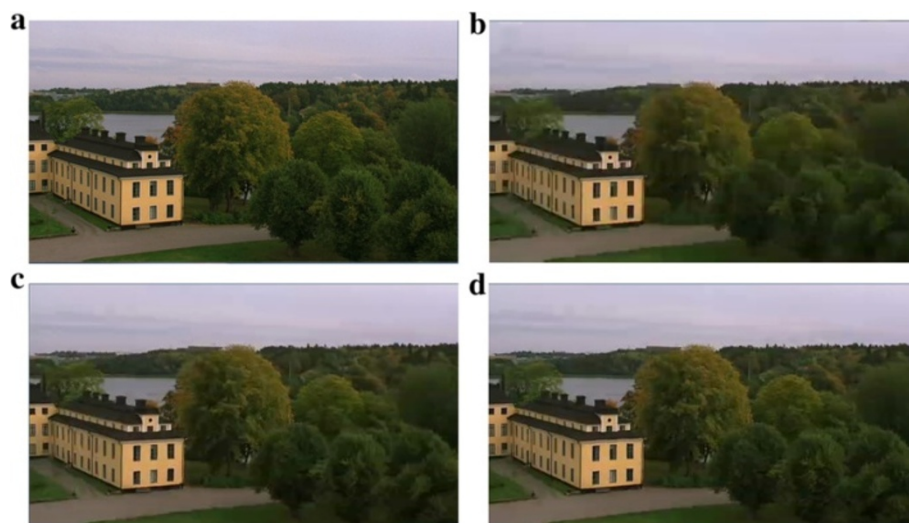
Figure 8 Subjective quality comparison of one 640 × 360 sequence. (a) Original frame of 'In_to_tree'; (b) 'In_to_tree' by MSE-ER (SSIM 0.833); (c) 'In_to_tree' by SSIM-ER [19] (SSIM 0.860); (d) 'In_to_tree' by our proposed (SSIM 0.873).
