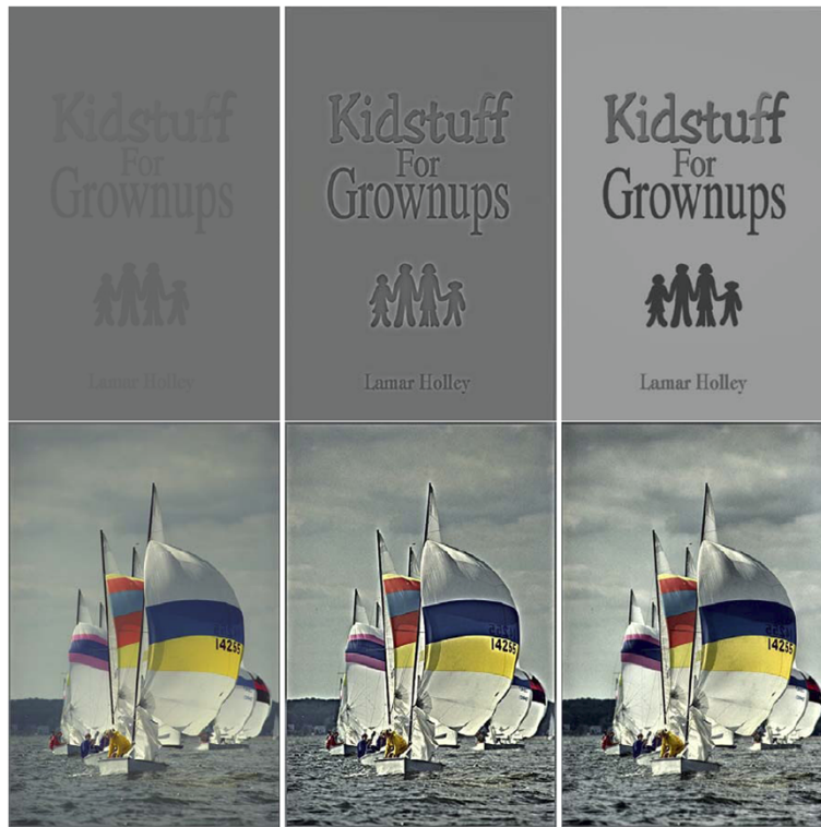
Figure 5 Image sharpening results. From the first to the third column are input image, results of conventional gradient domain method (Laplacian subtraction) in [10] and the proposed method.
