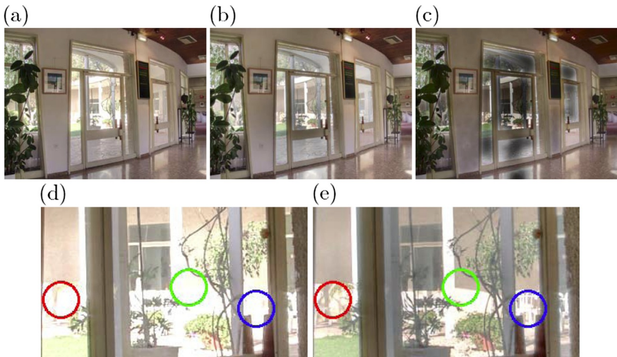
Figure 10 Comparison of conventional exposure fusion and the proposed method. (a) Result of exposure fusion [17]. (b) Result of the proposed method. (c) The result when the data weight is a constant. (d) Cropped image from (a). (e) Cropped image from (b).
