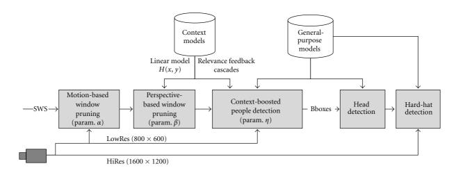
FIGURE 4: The scheme of the domain-specific video surveillance. The meaning and use of parameters  $\alpha$ ,  $\beta$ , and  $\eta$  are provided in Section 5.1. The use of multiresolution video data is described in Section 3.2.
