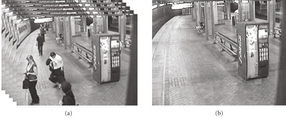
FIGURE 1: Typical example of estimating the background from a cluttered image sequence: (a) input frames cluttered with foreground objects, where only parts of the background are visible; (b) estimated background.
