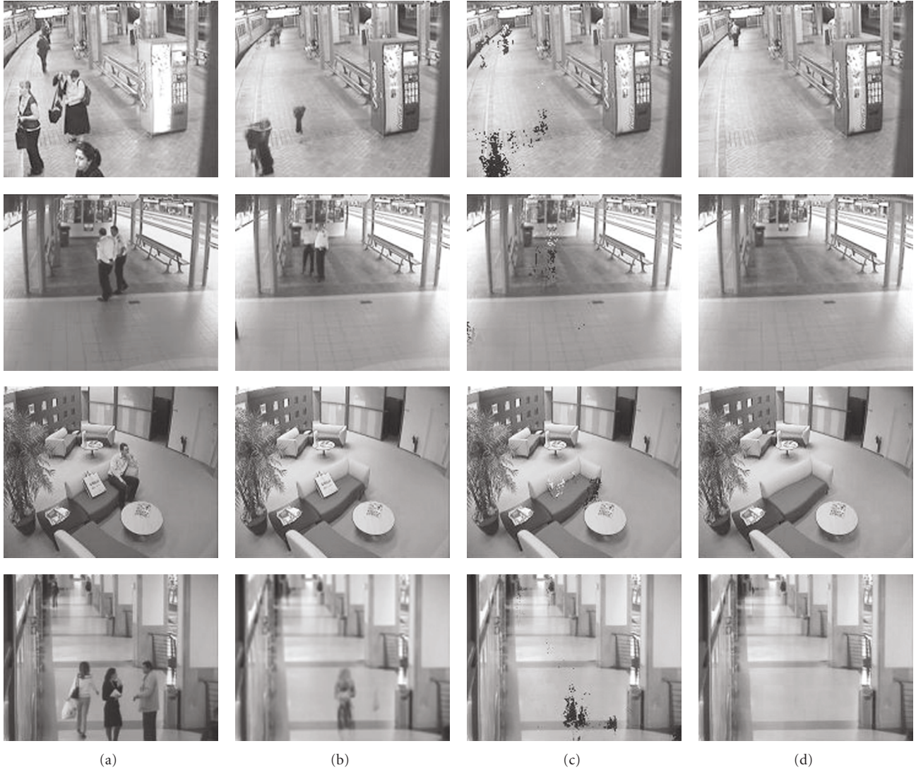
FIGURE 6: (a) Example frames from four videos, and the reconstructed background using: (b) median filter, (c) ISI method [14], and (d) proposed method.
