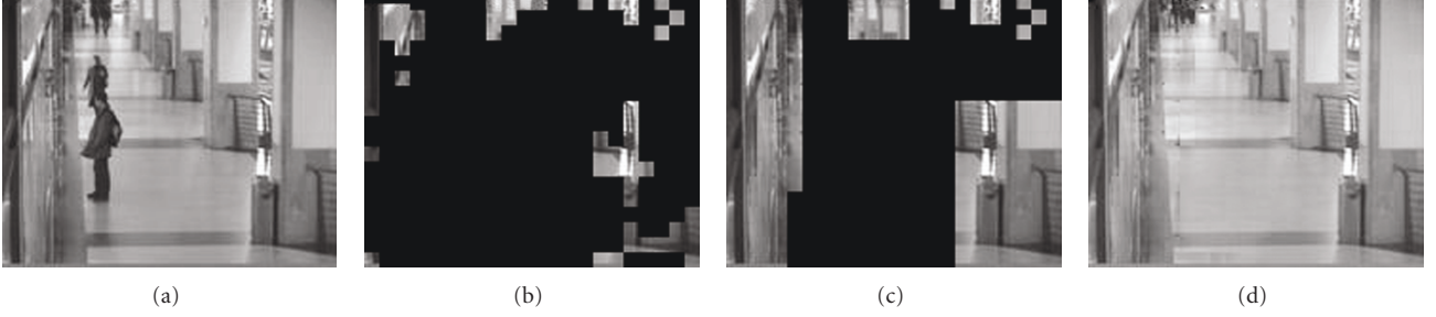
FIGURE 2: (a) Example frame from an image sequence, (b) partial background initialisation (after Stage 2), (c) remaining background estimation in progress (Stage 3), (d) estimated background.
