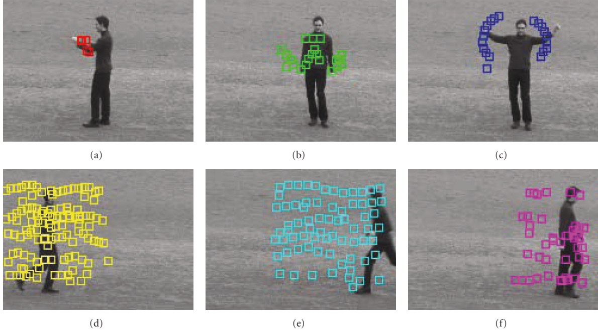
FIGURE 2: Sample sequences with detected interest points using the approach in Section 3.1 for the KTH dataset. From (a) to (f), the activities are boxing, handclapping, handwaving, jogging, running, and walking. Note that these interest points are detected at places where complex, nontranslational motions occur.
