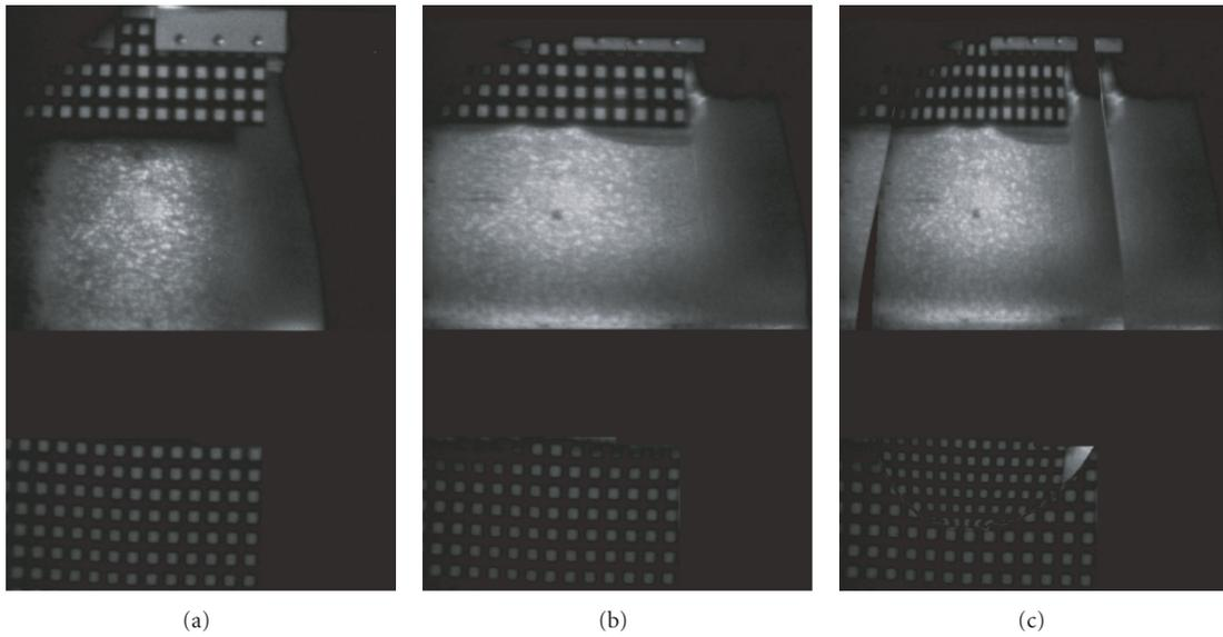
FIGURE 14: Illustration of the precorrection: (a) reference image number 13, (b) raw image number 24, (c) corrected image number 24.
