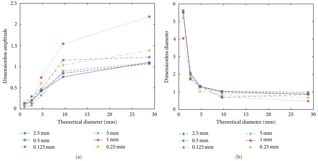
FIGURE 13: Estimated amplitude (normalized by the imposed one) versus diameter for different amplitudes (a). Estimated diameter (normalized by the imposed one) versus diameter for different amplitudes (b).
