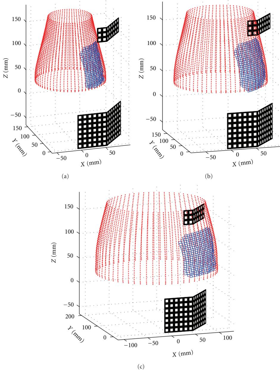
FIGURE 15: Reconstruction of the specimen surface at three stages of expansion, image no. 6 (a), image no. 13 (b) and image no. 25 (final one) (c). The deformed mesh represents the reconstruction data while the points represent the interpolated surface.
