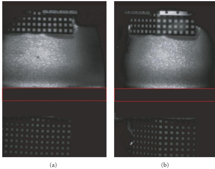
FIGURE 16: Last image pair (left and right views). On the lower part (inside the red rectangle), a necking appears.
