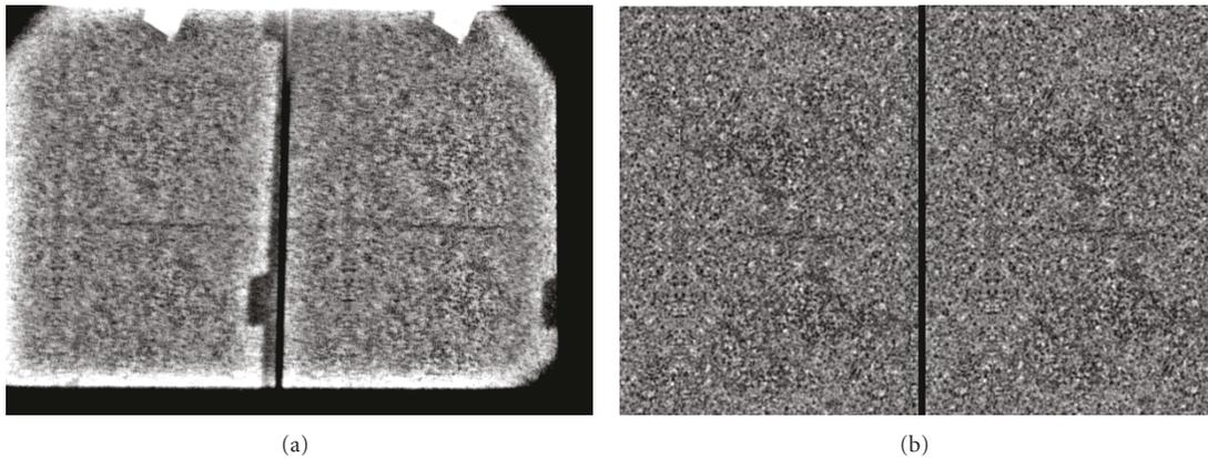
FIGURE 8: Images obtained with stereoscopic mirrors and used for estimating of distortions (a). The white rectangle located on the upper edge of the field corresponds to a piece of adhesive tape used to fix the calibration pattern onto the machine support. Digital images printed on the calibration plate (b). The distortions of the whole optical chain is assessed by registering the left and right parts of both pictures.
