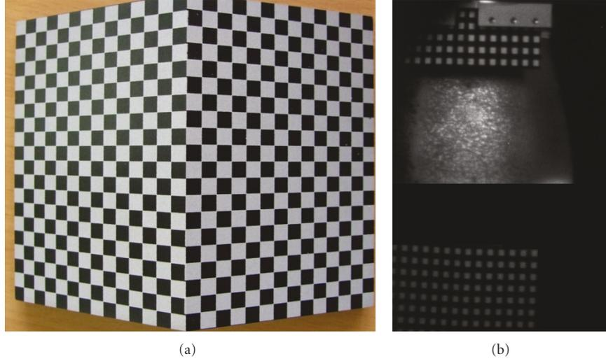
FIGURE 3: Calibration target (a) and its positioning on the experimental stage (b). The centers of the white squares are automatically detected after a local thresholding and a calculation of the barycenters of the detected related components. The calibration is performed by matching the image coordinate of those centers and their 3D counterparts.
