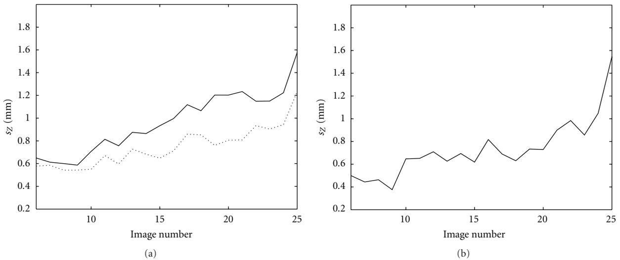
FIGURE 17: Evolution of surface roughness, evaluated over the entire surface or a central zone, total zone (plain curve), on a central zone (dotted curve) (a) and locally (b).
