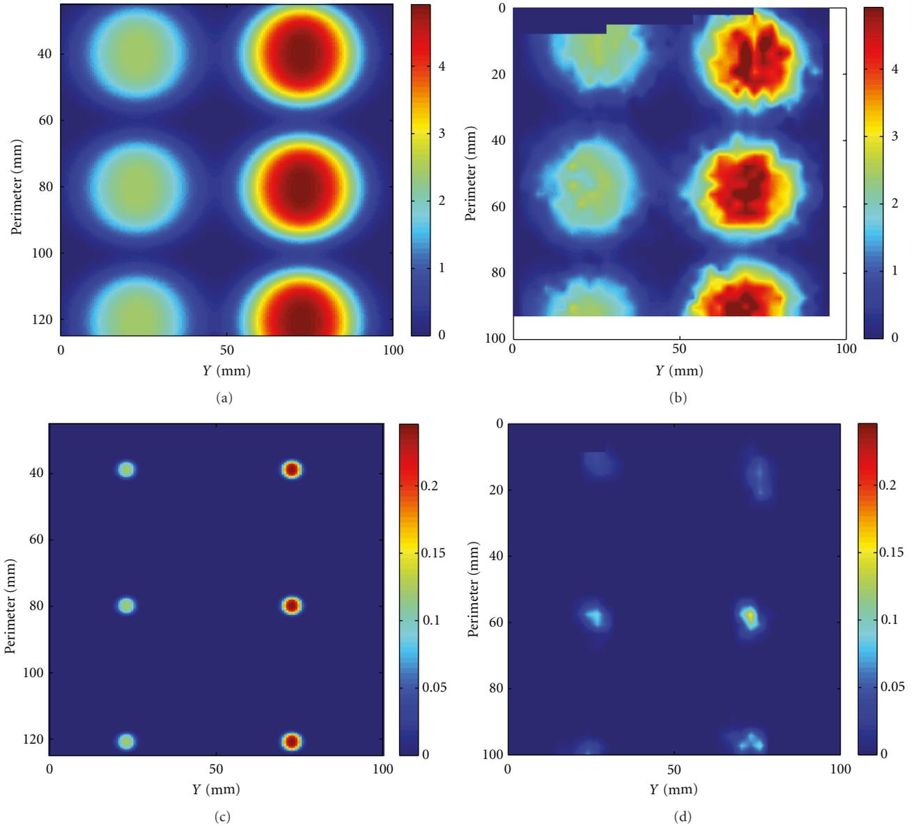
FIGURE 12: Comparison between the imposed (unfolded) surface displacement (left) and as determined from stereoreconstruction from synthetic images (right). The top figures show bumps of 30 mm diameter, and 2.5 mm, or 5 mm amplitudes. The bottom figures show bumps of 5 mm diameter, and 125  $\mu\text{m}$  or 250  $\mu\text{m}$  amplitudes.
