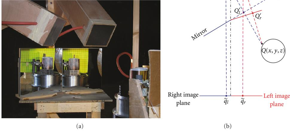
FIGURE 1: Visualization of the stereoscopic system (a). Reference mirrors in which the cylinder and the calibration target can be seen. Above the mirrors, the pyrotechnic flashes are located in wood cases. Model of image formation in the case of two mirrors of reference and with an orthographic model (b).
