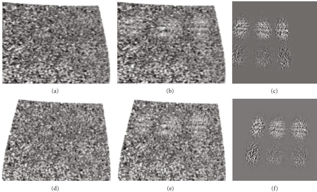
FIGURE 11: 3D surface rendering when unfolded onto a plane. Reference (a) and deformed (b) left images, and their difference (c). Reference (d) and deformed (e) right images, and their difference (f).
