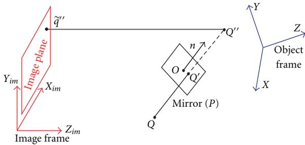
FIGURE 2: Model of image formation via a mirror  $P$  of normal  $\mathbf{n}$ .
