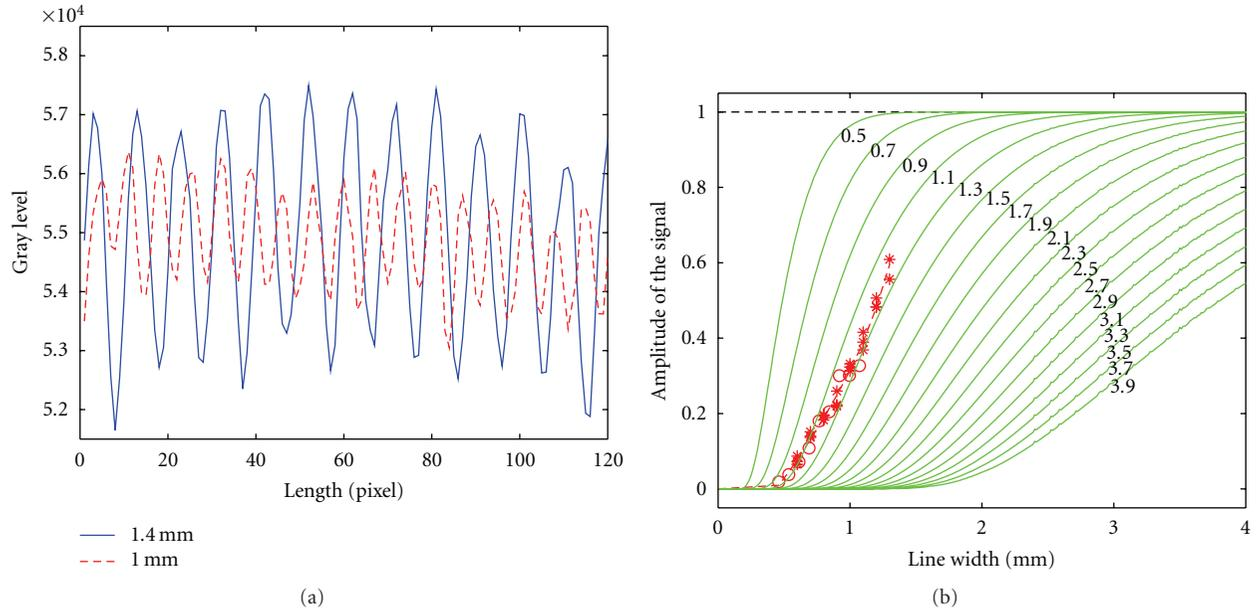
FIGURE 7: (a) Evolution of gray level contrast with the spatial period of the crenels. (b) Normalized contrast versus line width: experimental points (red symbols) and curves (green) obtained for a linear system with a Gaussian transfer function of varying FWHM from 0.5 to 3.9 mm.
