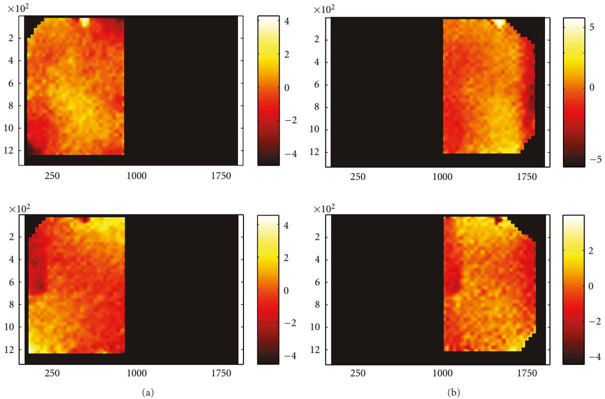
FIGURE 9: Measured distortion taking into account the stereoscopic mirrors, left (a) and right (b) mirrors. The color scale encodes the magnitude of the displacement expressed in pixel (1 pixel =  $180\ \mu\text{m}$ ). The top (resp., bottom) figures show the displacement component along the longitudinal (resp., transverse) axis.
