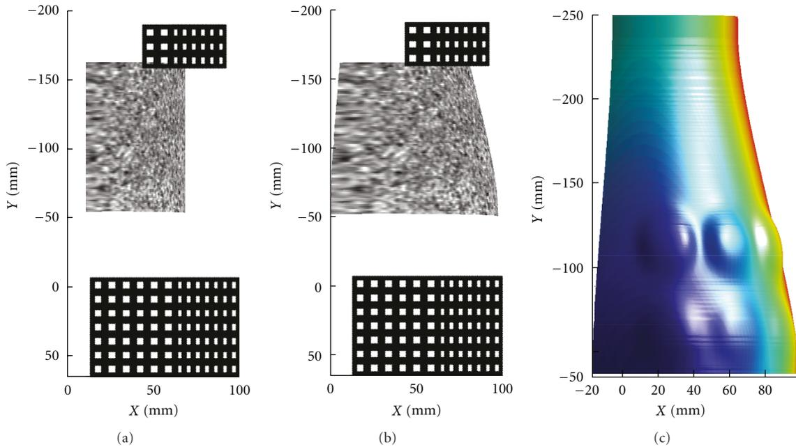
FIGURE 10: Reference configuration created by mimicking laser marking (a), deformed surface with a known displacement field (b). Addition of local bump defects on the deformed surface (c).
