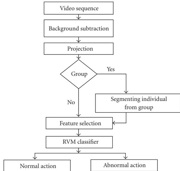
FIGURE 1: The block diagram of the Video Surveillance System.
