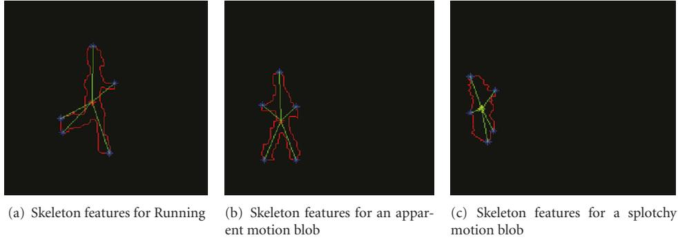
FIGURE 8: Skeleton features for different motion blobs.
