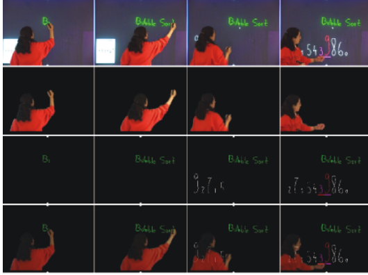
FIGURE 4: The approach presented in this article (images created using the algorithm presented in this article). The remote listener watches a remote lecture where the extracted lecturer is overlaid semitransparently onto the dynamic board strokes which are stored as vector graphics. Upper row: original video; second row: segmented lecturer video; third row: board data as vector graphics. In the final fourth row, the lecturer is pasted semitransparently on the chalkboard and played back as MPEG-4 video.
