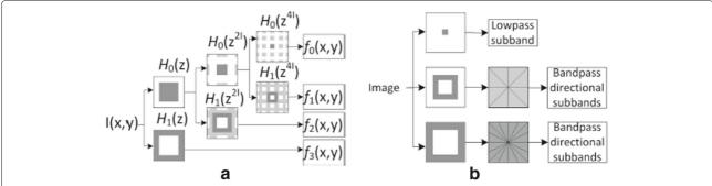
Fig. 1 Non-subsampled contourlet transform. Non-subsampled contourlet transform for (a) three-stage pyramid decomposition. (b) Non-sampled filter bank
