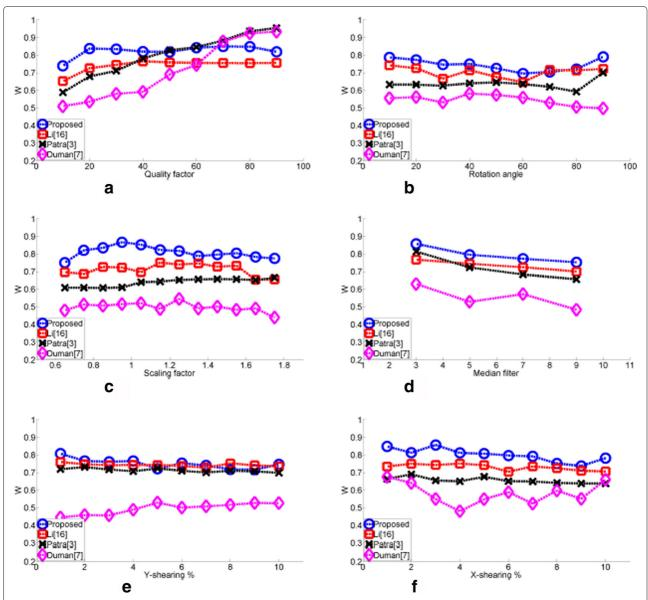
**Fig. 9** The maximum NHS comparison among various attacks for Lenna image. Results for JPEG compression, rotation attacks, scaling attacks, median filter, and *Y* and *X* shearing percentages of the proposed approach in comparison with Li [27], Patra [7], and Duman [11]. **a** JPEG compression. **b** rotation attacks. **c** scaling attacks. **d** median filter. **e** shearing Y %. **f** shearing X %
