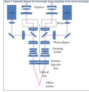
The stereo microscope can be analyzed like stereovision because of the two slightly different optical paths about one object. Figure 4 shows the schematic diagram for the stereovision analysis part at the optical structure of the stereo microscope. The CCD is assumed to be the coordinate system;  $\vec{a}$  and  $\vec{a}$  represent the points which are the object position  $\vec{a}$ . The distance  $\vec{a}$  is estimated by the stereovision method as follows:
